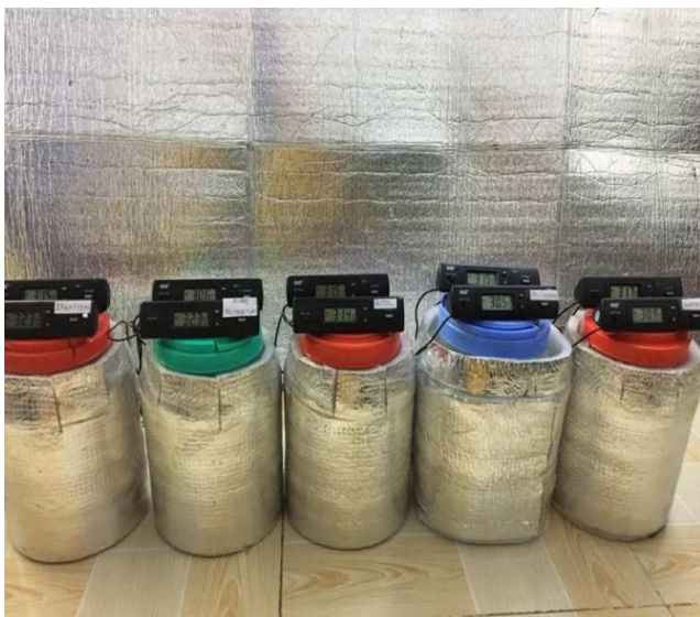
Figure 3. The picture of experimental process of discharging for phase change materials.
