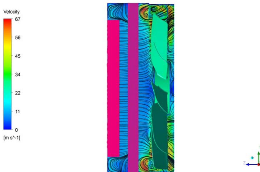
Figure 2. Three-dimensional flow field of cooling module with serial structure.
